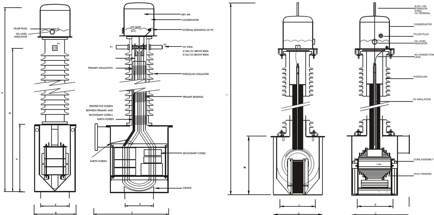
STANDARD DIMENSIONS (mm) for single phase post type current transformers: 22kV - 132kV
